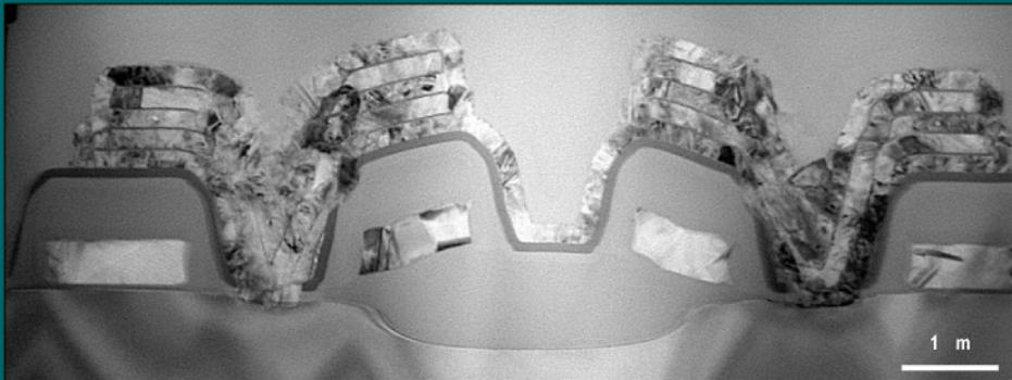
1. Cross-sectional TEM image of an IC device.
