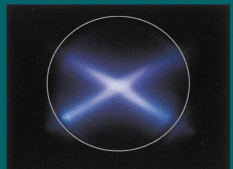
View of the fluorescent screen through the viewing window showing the ion beams intersecting at the center.
