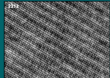
8. High resolution TEM image of  $T_C$  superconductor (2212) milled in the PIPS.
