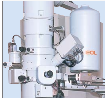
External view of the JEM-2100 with the JED-2300T and GUI for EDS analysis.
