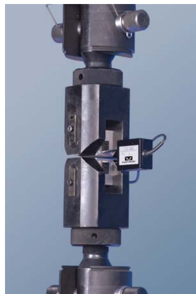
▲ A COD gauge is used to measure crack opening displacement during a fatigue crack propagation test
