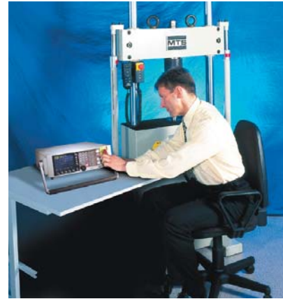
▲ Non-Instron frames that have been upgraded with FastTrack 8800 controllers
