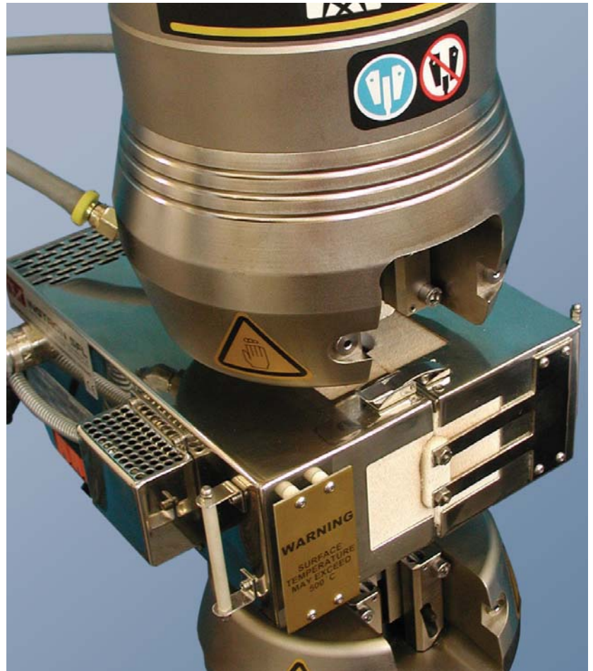
▲ +1400 °C short furnace and water-cooled hydraulic grips
