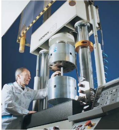
▲ Non-Instron frames that have been upgraded with FastTrack 8800 controllers
