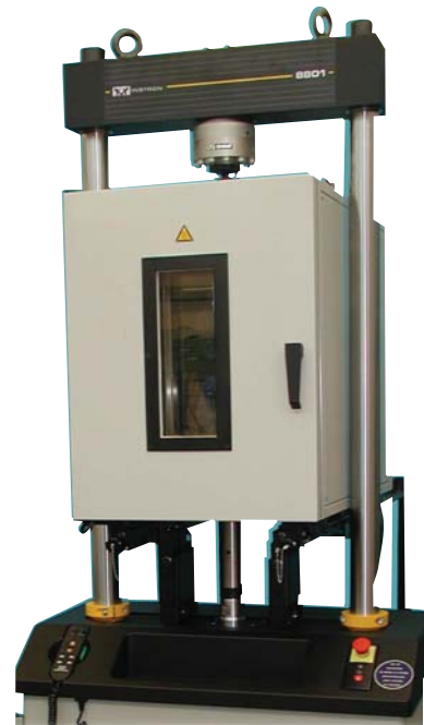
▲ Environmental chamber mounted on an extended height 8801 machine
